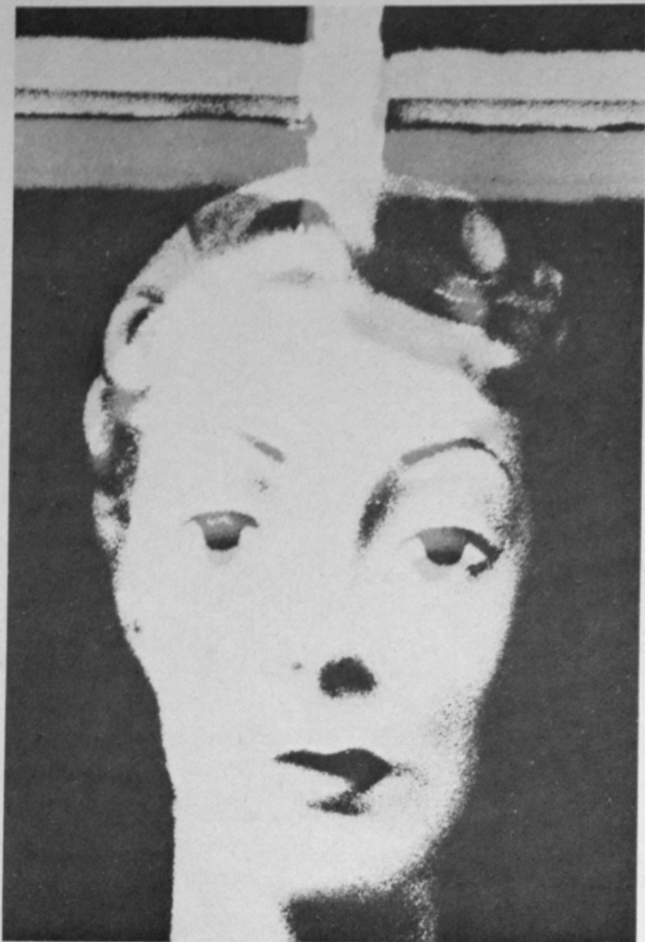
Figure 13. Superimposed enlarged transparencies of a manikin head on-axis and off-axis reveal differences in shape.
