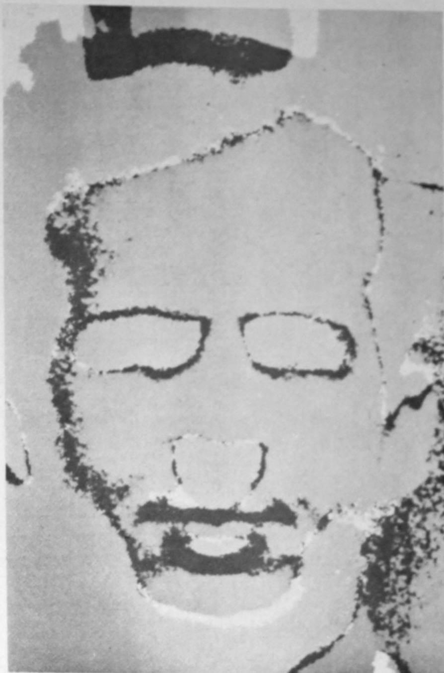
Figure 11. A high-contrast green negative image from one view combined with a high-contrast magenta positive image from another view reveals the areas of disparity vividly. (Original in color.)
